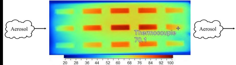
Figure 4. Sample thermal image of optimized-16cm heating section with control base module regulating thermo-couple temperature to 70°C under high flow nasal cannula therapy conditions
