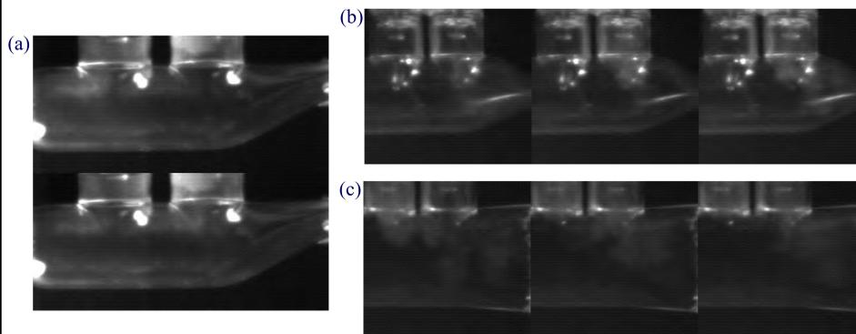
Figure 2. Frame montage of aerosol production and movement in clear prototyped devices a) Initial device, b) Optimized device, and c) Vertical-Optimized device
