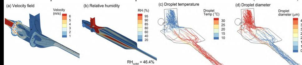
Figure 5. CFD assessment of the initial-12-cm design including selected mid-plane contours of a) velocity magnitude and b) relative humidity (RH), as well as droplet trajectories contoured based on c) droplet temperature and d) droplet/particle diameter
