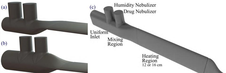
Figure 1. Air flow pathway of a) Initial-12-cm, b) Optimized-16-cm, and c) Vertical-Optimized-16cm designs intended to provide aerosol depositional losses <5%, submicrometer outlet particles, and an airstream comfortable for continuous direct nasal inhalation.
